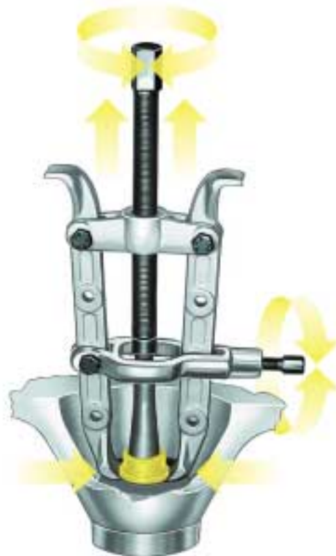
How a two arm puller works
