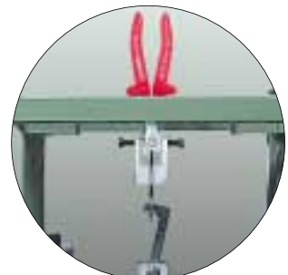
Testing adherence of the PVC coatings
