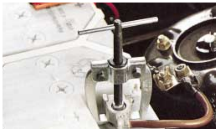
Battery terminal puller in use on a car battery
