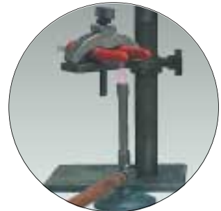
Testing resistance to fire
